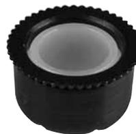
This bushing is pressed into the Trip Casting and is key to proper operation of the trip components on the Distributor. Keep this bushing pressed squarely into bolt-type Casting 090 006 665 or old roll pin type Casting 070 006 667.
