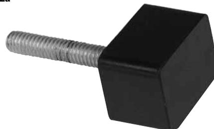
Goes through Sweep Stabilizer (top) Link 070 003 238. During regular inspection, or if your sweep "pops" when it starts down, make sure these are the correct thickness and not sticky. It is a direct replacement for obsolete rubber bumper 000 023 216.
