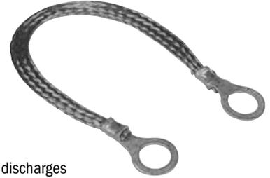
This discharges static electricity that would otherwise build up in the bounce plate assembly. If your scoring system freezes or locks up, inspect to make sure this strap is present, intact, and connected properly.
