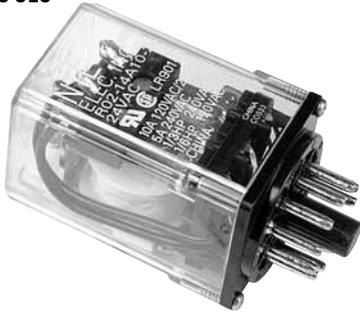
The common "ice cube" relay in most chassis. In the SS chassis, SP relay 070 005 883 looks very similar, but it has a 10 VCC coil and is not interchangeable.
