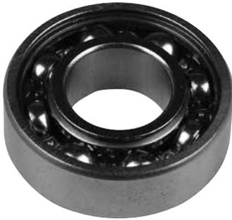
The rotor shaft inside every motor is supported at the end by one of these bearings. Don't let a questionable bearing ruin good endbells and rotor shafts. Bearings that don't feel smooth or turn with even resistance should be replaced.
