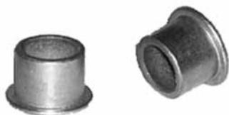
The heart of the LBS, this bushing is used extensively in the mechanism to ensure reliable operation. The Light Ball Sensor is intended to run perfectly clean and dry. No lubrication should be added to any parts in this assembly.
