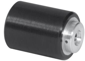
Two of these wheels protrude from the bottom of the lane machine to move it up and down the lane with minimal effect on the lane conditioning pattern. Replacing old A0994 and A0995 wheels, these are bidirectional and handle heavy oil conditions better than older versions.
