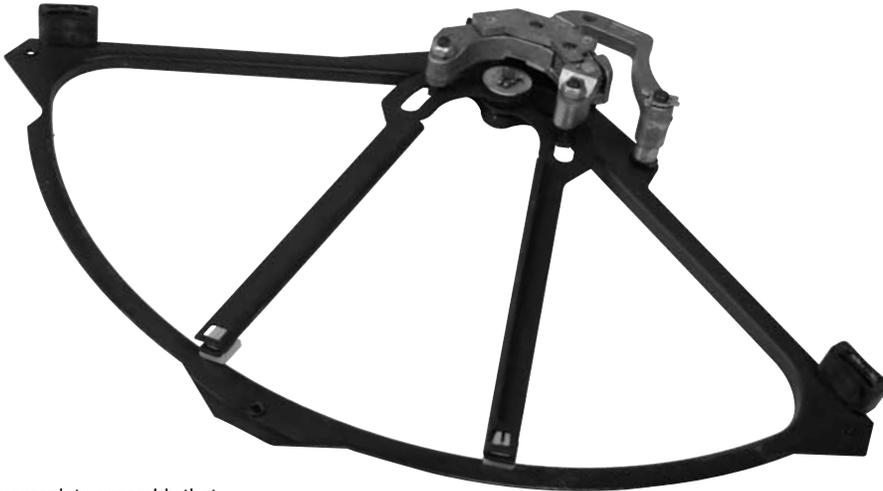
The complete assembly that picks up each standing pin while fallen pins are swept away. Used for pins #1-6 and 8-10. The #7 cell is different from the rest, and there are two different versions of the #7 cell. Early 82/70's with long carb link use #7 Cell 070 007 199. Most have a bolt connection at the #7 cell and use the 070 006 674.
