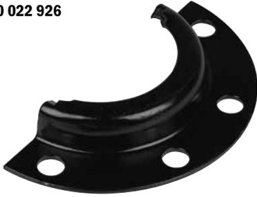
Direct replacement if the Rear Roller Bearing Support breaks on the ball door side. Remove old part, drill holes if necessary and secure with 810 258 100BG screws and 844 058 002BG nuts.
