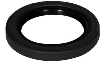
If a groove is worn in an output shaft from the old seal, a new seal can usually be seated slightly further in than the old one to contact a new area on the shaft and prevent leakage.
