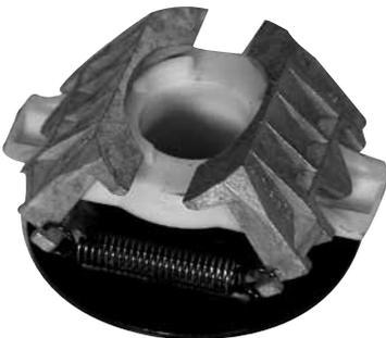
The "wide disk" mechanism and switch for starting late model Westinghouse and A.O. Smith BE motors. This type of centrifugal mechanism is held in place on the rotor shaft with clips on top and bottom. Match your rotor shaft to the appropriate mechanism type before ordering.
