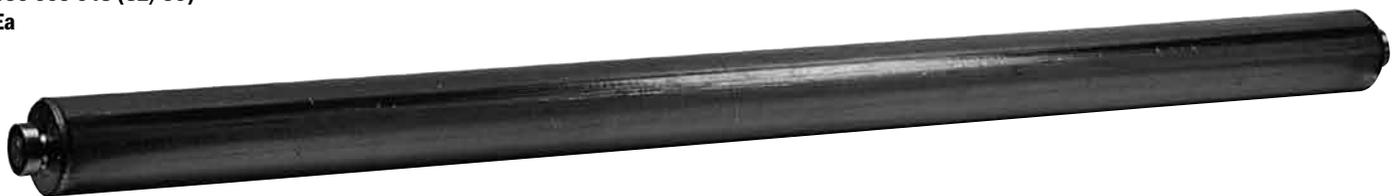
At the back of the pit, this roller drives the carpet belt. If the pulley is frozen on the shaft, loosen setscrews and start/stop BE Motor until pulley spins free.
