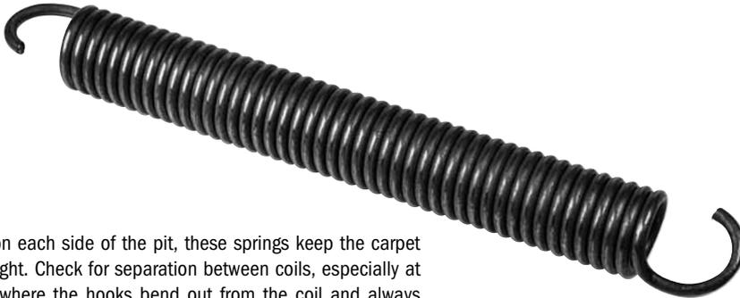
One on each side of the pit, these springs keep the carpet belt tight. Check for separation between coils, especially at ends where the hooks bend out from the coil and always replace these springs in pairs. Some mechanics find it easier to stretch the spring into place on the back post using a 2' length of 1/2" dia. conduit as a lever.
