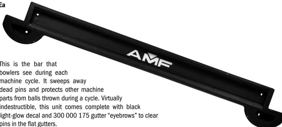
This is the bar that bowlers see during each machine cycle. It sweeps away dead pins and protects other machine parts from balls thrown during a cycle. Virtually indestructible, this unit comes complete with black light-glow decal and 300 000 175 gutter "eyebrows" to clear pins in the flat gutters.
