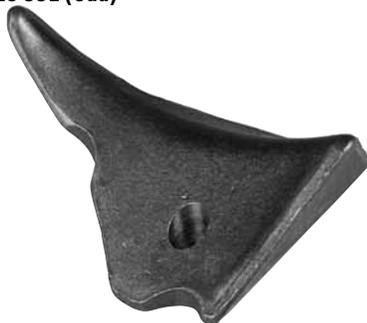
Seven required per pinspotter to hold pins in the pin elevator. If pins are sticking in the wheel and going past the distributor, clean the wheel surface and check these for wear.
