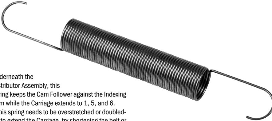
Underneath the Distributor Assembly, this spring keeps the Cam Follower against the Indexing Cam while the Carriage extends to 1, 5, and 6. If this spring needs to be overstretched or doubled-up to extend the Carriage, try shortening the belt or cleaning and repacking bearings in the 070 006 011 belt rollers.
