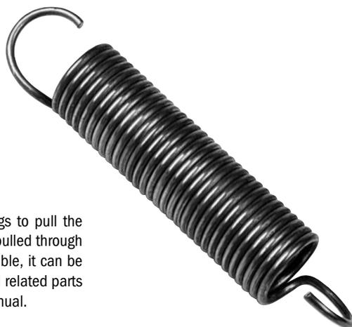
Steel tables use two of these springs to pull the yoke forward. If the spring stud has pulled through the table casting on an aluminum table, it can be replaced by two of these springs and related parts as shown in any steel table parts manual.
