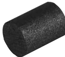
Four of these drag on a disc in National combination motors to add resistance for braking.
