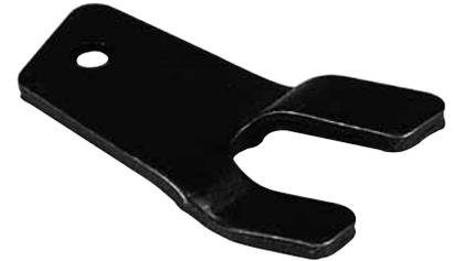
Bolted to the Trip Casting, this part engages the clutch to index the distributor when tripped. If these are binding, the contact surfaces may need to be greased, or may have changed shape from wear.
