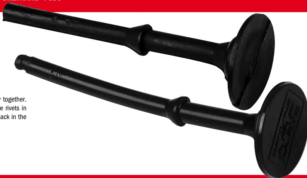
16 of these hold the cushion assembly together. Some mechanics install heavy-duty blue rivets in the high-wear positions and standard black in the others.
