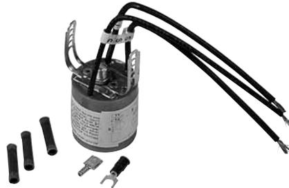
The length of time that the start winding is engaged can be adjusted with this type of solid state start switch. Often known as the "Lewus" switch, this is not recommended for combination motors.
