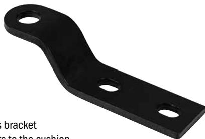
This bracket bolts to the cushion hanger weldment and attaches it to the bottom ring of the shock absorber. Keep these bolts tight and make sure the hole for Pin 000 022 821 is round and keeps a snug fit.
