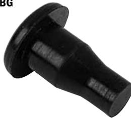
Used to cushion moving parts all over the Distributor, this small bumper can also be found in the PBL Ratchet Crank, behind the Bin Switch Lever, and under the Spotting Solenoid on 82/70's. Washer 948 767 132BG can be sandwiched under the bumper head to adjust the stopping position of moving parts if necessary.
