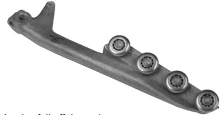
As pins fall off the end of the distributor, they push down these arms and advance the distributor to its next position. Bearings that are missing or that don't spin freely should be replaced with Bearing 000 026 251BG, Screw 813 540 082BG, and Lockwasher 957 100 002BG.
