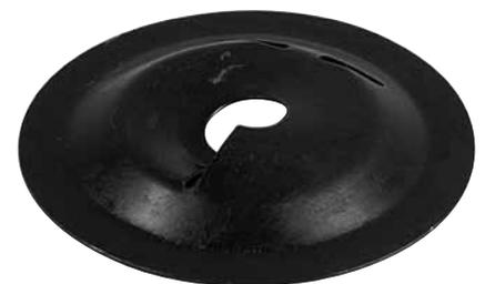
This is the constantly rotating part of the Clutch. Adjusting spring rotation determines its pressure against the friction disc. To ensure proper operation, the friction surface on this plate must be completely flat, and the opening must screw neatly onto the worm. You can check these by looking for air gaps when you set the plate on a flat surface and when you stack it with another plate.
