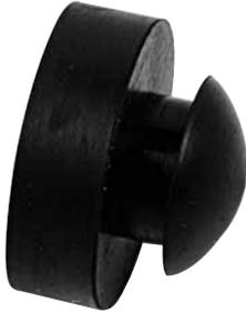
Most commonly used for protecting pins in the Bin assembly, this bumper is also for the start switch lever, and for closed pinwheels on early 82/30's. Made of 100% neoprene rubber for best performance. File off any sharp metal edges around mounting holes prior to installing. Twist them as you press them into place. Some mechanics use a drop of liquid dishsoap on the round surface to help ease installation.
