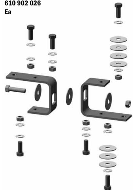
If the back end of a machine migrates away from the front end, it can crack the brackets where the two machine halves meet. Use this kit to repair the damage, and make sure that Floor Bracket 000 026 464 is mounted firmly at both rear corners of the machine.
