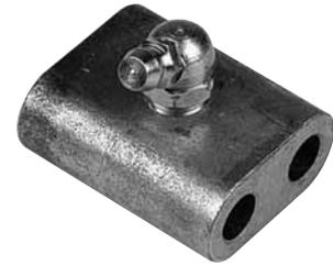
This is what pivots between the two halves of the Front Roller assembly. When assembling, make sure grease zerks point toward the hole in roller body. Interested in trying the lube-free plastic version? If so, order 000 024 760. Always replace these in pairs.
