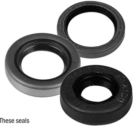
These seals prevent leakage around the four gearbox shafts. When installing, prevent seal damage by wrapping sharp edges on shafts with teflon tape and coating shafts with gearbox oil.
