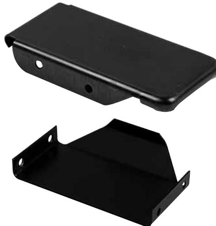
These are located throughout the Bin Assembly and locate each pin as it falls in from the Distributor. When replacing, hold the mounting face of Shock Mount 070 006 354BG tight against the butt guide as you tighten the screws. This helps prevent twisting during installation and premature failure.
