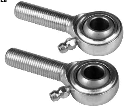
Used in tie rod assemblies on the Sweep and Table so adjustments can be made by turning the tube. Includes grease zerk for easy maintenance. Secure with Jam Nut RH 835 570 002BG or LH 835 670 002BG.
