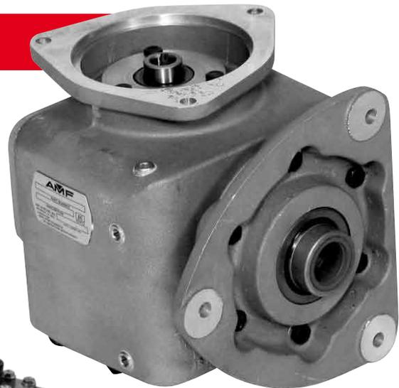
Two of these gearboxes mount to the front end of the machine to run the sweep and the table. Clean output splines while gearbox is off of pinspotter and apply grease prior to installation. The splines will wear longer and it will be easier to remove the gearbox in the future.
