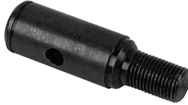
If a front roller pivot stud is worn out, break it out of the kickback plate with a large wrench and replace it with this. File/grind/chisel old weld as necessary to position new stud perpendicular to plate, then secure tightly with 844 074 002BG Nut and 941072200BG washer.
