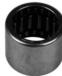
The key to either machine on a pair being able to run the shared ball lift, this clutch bearing locks when turned one direction, and freewheels in the other. This is the same bearing used on the lower shaft of AMF-type front ball returns including C-90, Options and Profile.
