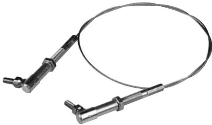
As pins push down the trip arms when they're leaving the distributor, this cable trips the rocker arm and begins the index to the next location.
